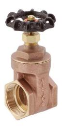
Grit, dirt or any foreign matter accumulated in the pipe can hinder the efficient valve operation and seriously damage vital valve parts. Thoroughly clean pipe with air or steam or water and make sure waterway is clear.
